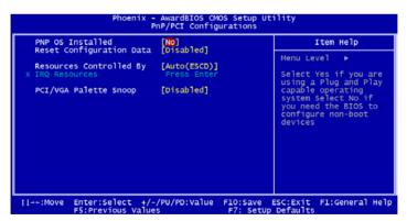
Figure 3.10: PnP/PCI configurations screen
